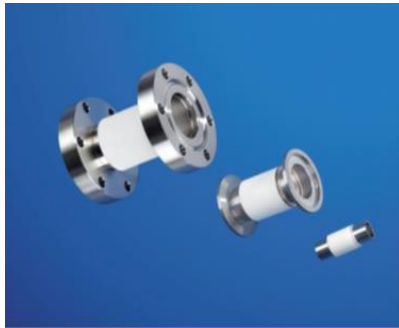
Kicker tube of a particle accelerator, consisting of externally copper-plated Al_2O_3 with brazed metal flanges on the front edge.
